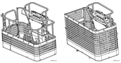
Figure 19. Fabric Mesh to Mid Rail
