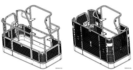
Figure 22. Platform Mesh to Mid Rail
