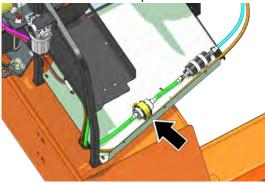
Fuel Filter (Propane) Interval - 3 Months or 150 hours of operation Comments - Replace filter.
