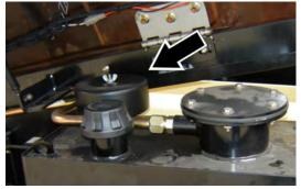
Wheel Drive Hub Lube Point(s) - Level/Fill Plug Capacity - 24 oz. (0.8 L)(1/2 Full) Lube - EPGL Interval - Check level every 3 months or 150 hrs of operation; change every 2 years or 1200 hours of operation
