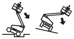
Do not elevate platform or drive with platform elevated while on or near a sloping, uneven, or soft surface.
