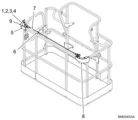
Figure 15. Bolt-On External Fall Arrest System
