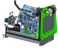
Fuel Pre-Filter - Deutz D2.9 L4 Lube Point(s) - Replaceable Element Interval - Drain water daily; Every year or 600 hours of operation
