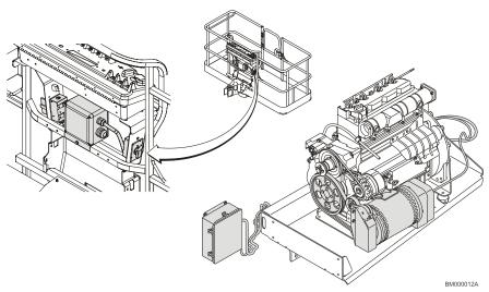
Figure 27. SkyPower and Generator Systems
