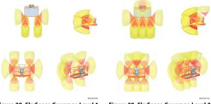
Figure 28. SkySense Coverage Level 1 Areas (2– Bar)
