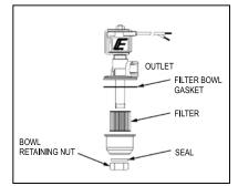
Figure 33. Kubota Filter Lock Assembly
