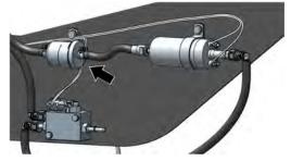
Fuel Filter (Propane) - Kubota Interval - Every year or 1000 hours of operation Comments - Replace filter. Refer to Section — Propane Fuel Filter Replacement (Kubota Engine)
