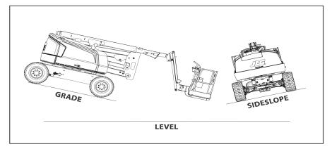
Figure 8. Grade and Side Slope
