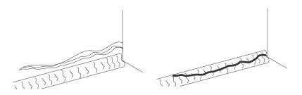
Figure 2. Parent Metal Crack
