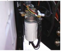
Fuel Filter - Deutz D2.9 L4 Lube Point(s) - Replaceable Element Interval - Every year or 600 hours of operation
